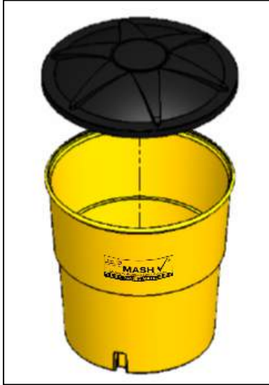
Figure 8a: 1400 lbs. Barrel Assembly.
