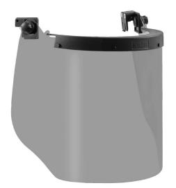
Full face protection that enables the wearer to work on or be in the vicinity of live parts with arc protection up to 10.0 cal/cm<sup>2</sup> (ASTM F2178-12). Recommended for use with balaclava. Securely flips up and down. Attaches directly to the 30 mm EURO Slots.
